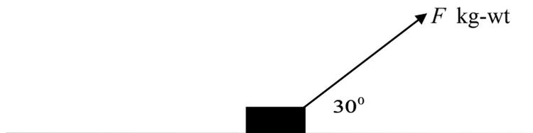
A box of mass 3 kg is on a horizontal plane. A force of magnitude  $F$  kg-wt acting at an angle of  $30^\circ$  to the horizontal is applied to the box. The coefficient of friction between the box and the plane is  $\frac{\sqrt{3}}{2}$ . Which of the following is true?
